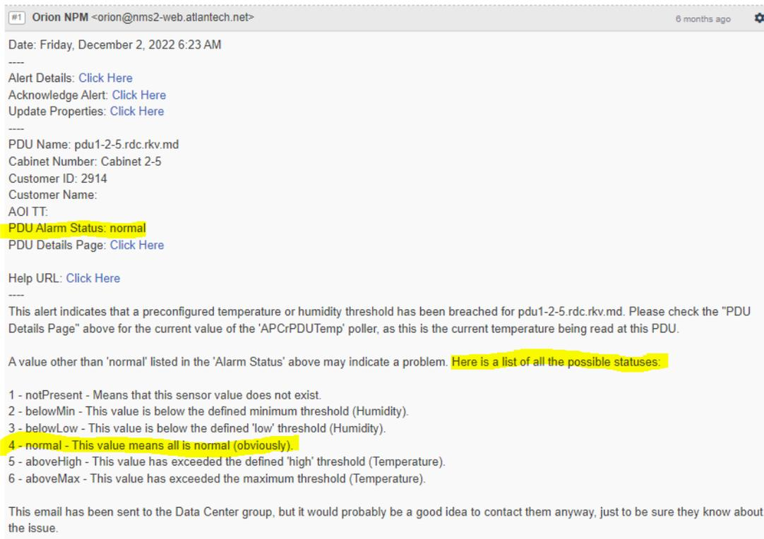
Look up what it means in the list of all the possible statuses in the above screenshot. In this example, the status “**normal**” means that the temperature and humidity values measured in the aisle are good. (This unnecessary alarm will pop up when Orion reboots, for example).
